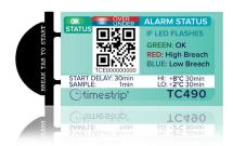
The Electronic Timestrip Complete TC 490 is a temperature indicator for the range 2°C to 8°C (36°F to 46°F). It uses a set of three LEDs to provide a clear, non-reversible indication of upper and lower temperature breaches as well as normal operation. The TC 490 is part of the eTimestrip product range.
